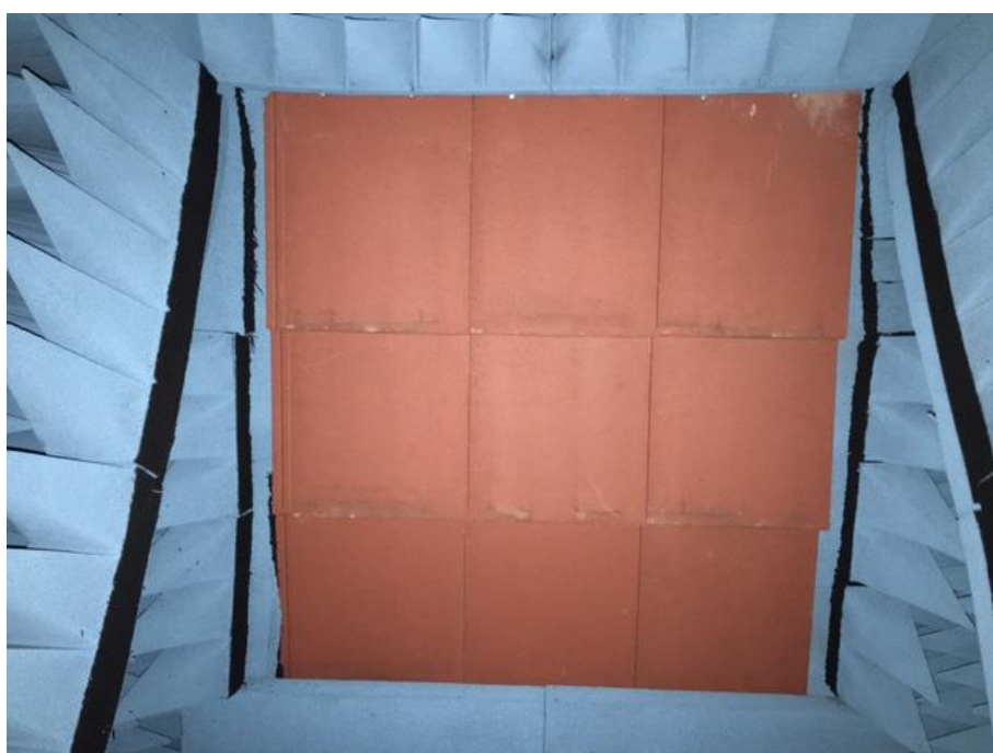
Figure 9: Test Frame containing Roofing material in position for testing
