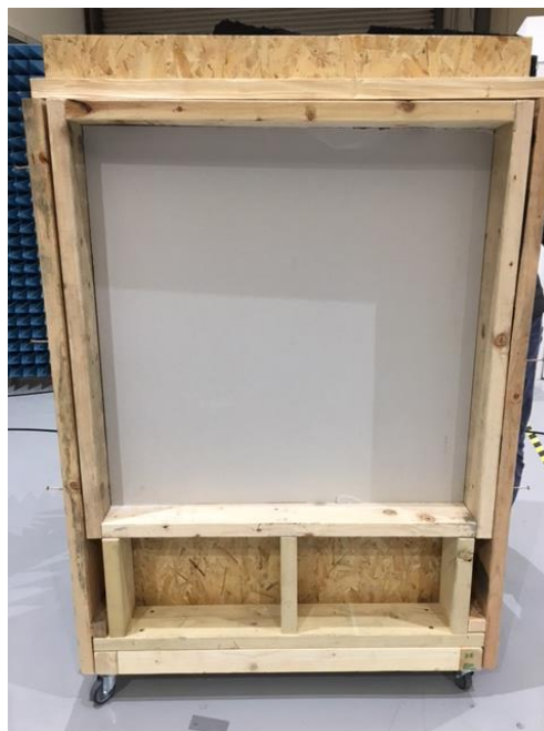
Figure 4: 1-by-1m wooden Test Frame with plasterboard insulating material mounted on a wheeled base
