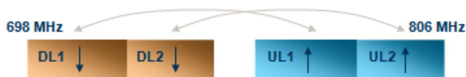
Figure 4. A solution with dual duplexers having the same duplex distance that could be of same or different sizes (DL1 paired with UL1 and DL2 paired with UL2)
