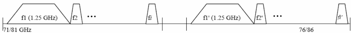
Figure A3.4: Example of aggregating multiple 250 MHz channels, possibly alongside with original 250 MHz wide channels within the single band 71 - 76 or 81 - 86 GHz
