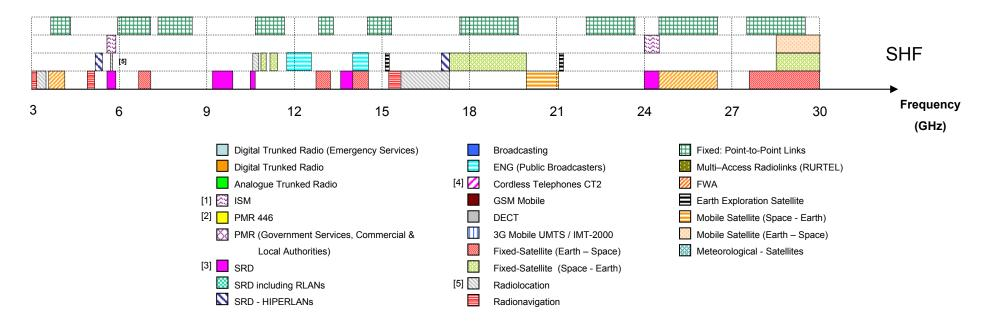
Note: This chart provides a representative overview of frequency allocations and usage in the UHF and SHF ranges. For clarity, not all services or uses are shown.
