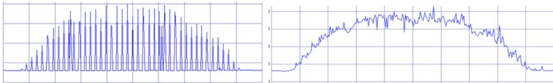
Figure 33 - Fragmented single after single sweep (left). Coherent signal after multiple sweeps (right)
