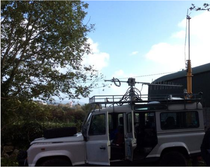
Figure 3.2: Vehicle at 'Ridge' site, test antenna at 5.2m, radar visible in background
