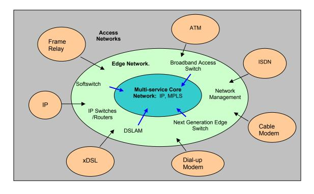
ATM: Asynchronous Transfer Mode IP: Internet Protocol DSLAM: DSL Access Module ISDN: Integrated Services Digital Network MPLS: Multi Protocol Label Switching DSL: Digital Subscriber Line.
