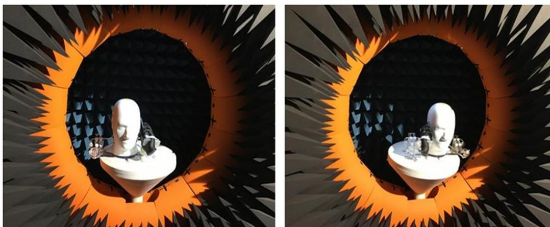
**Figure 3: Handset Positioning for BHHL (left) and BHHR (right) scenarios**
