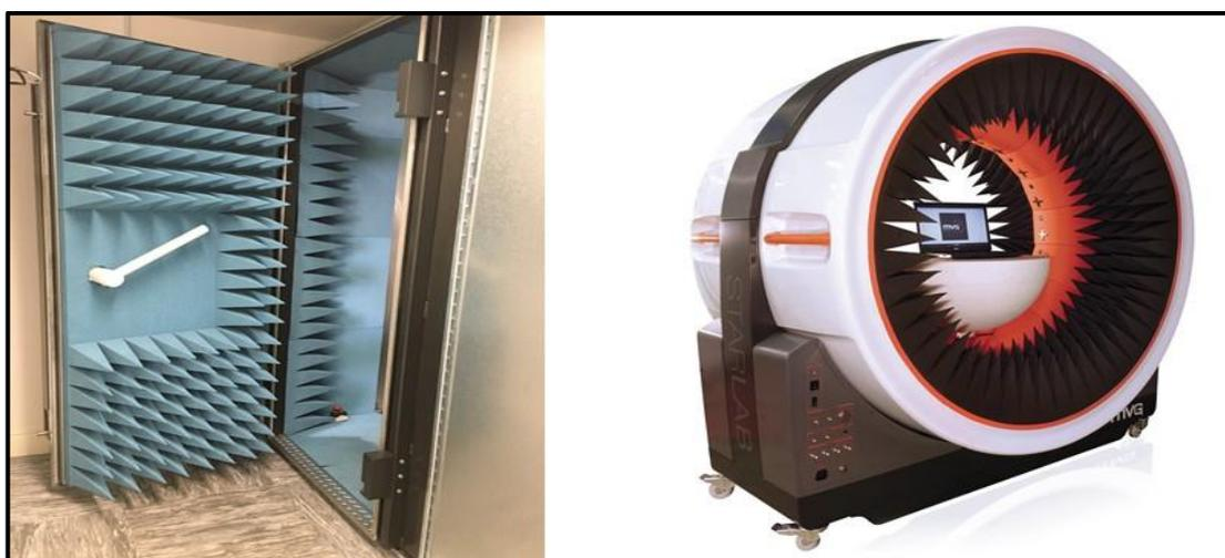
**Figure 2: MVG StarLab Measurement System on the right was placed inside the Anechoic Chamber on the left for TRP and TIS Measurement<sup>29</sup>**
