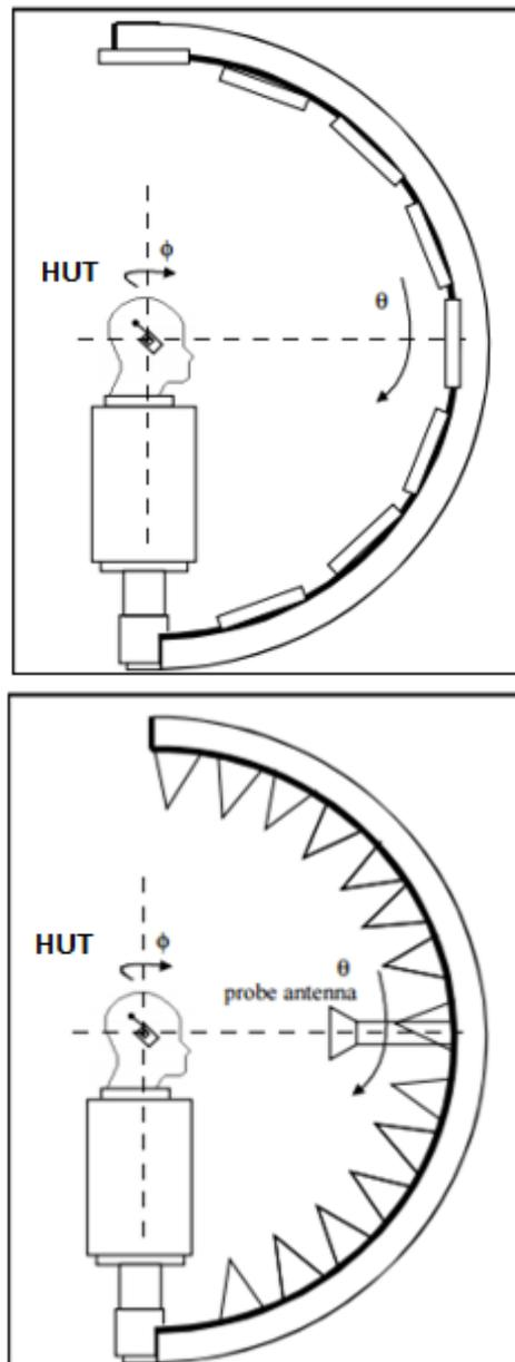
Figure 6: (a) Multi Probes (b) Single Probe (for illustration purpose)
