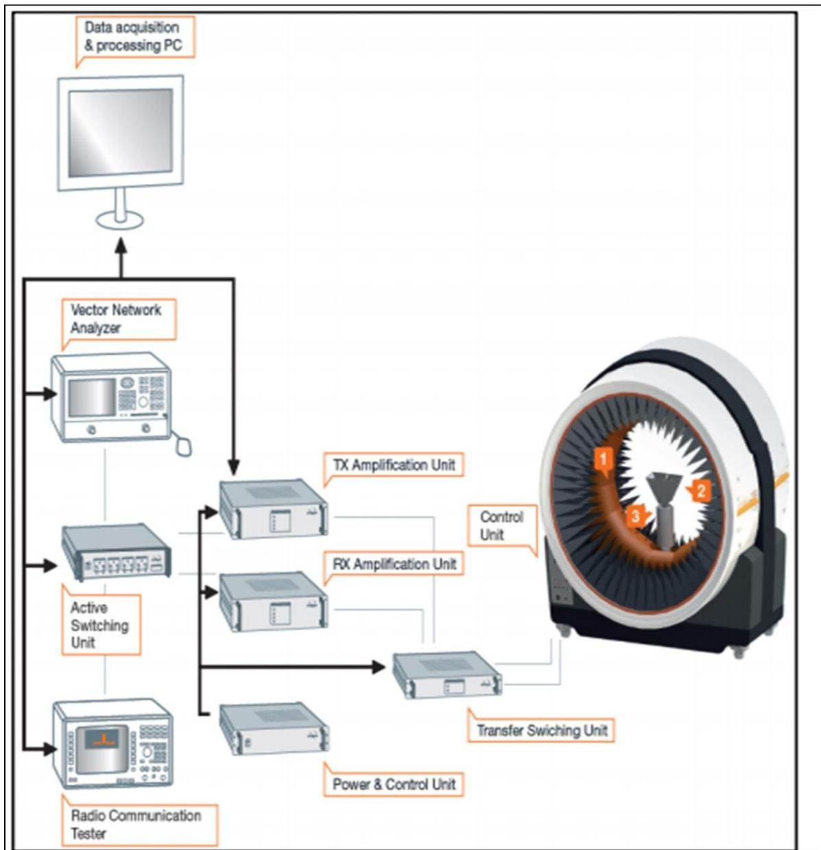
Figure 9: StarLab Test Setup<sup>45</sup>
