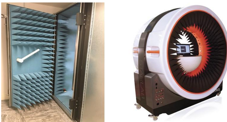
Figure 1: MVG StarLab Measurement System on the right was placed inside the Anechoic Chamber on the left for TRP Measurement
