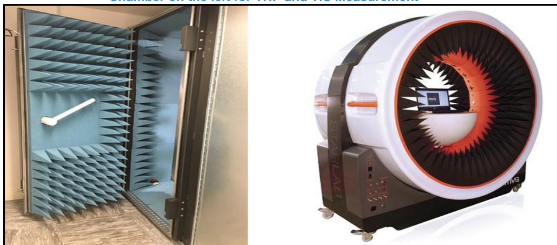
Figure 2: MVG StarLab Measurement System on the right was placed inside the Anechoic Chamber on the left for TRP and TIS Measurement 26
