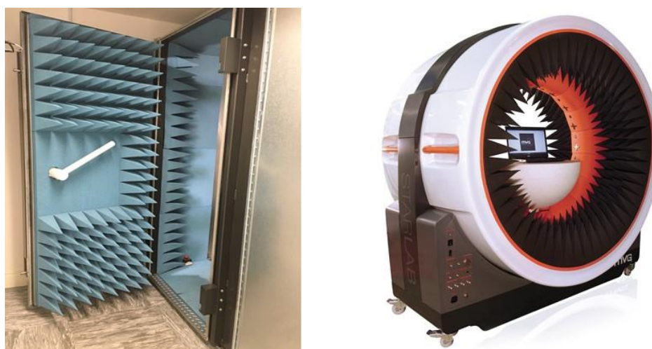
Figure 1: MVG StarLab Measurement System on the right was placed inside the Anechoic Chamber on the left for TRP and TIS Measurement
