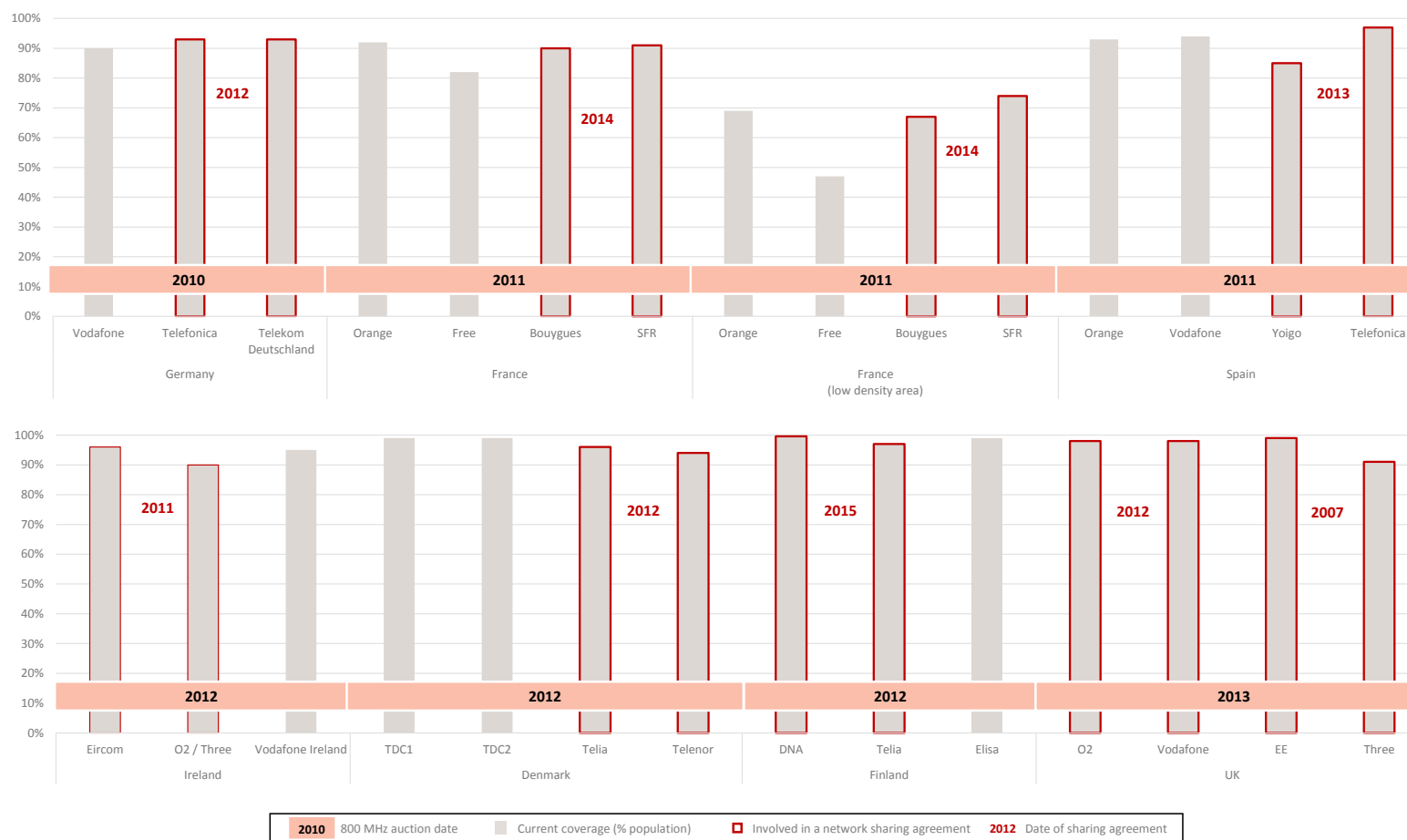
Figure A4.32 4G mobile network sharing agreements and 4G coverage by MNOs in selected countries (using most recent available coverage data from MNO websites, typically 2016–17)
