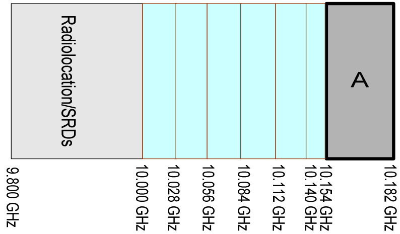
Figure 6: Suggested band plan with 28 MHz channels, and one 14 MHz channel/guard band at 10.140 – 10.154 GHz
