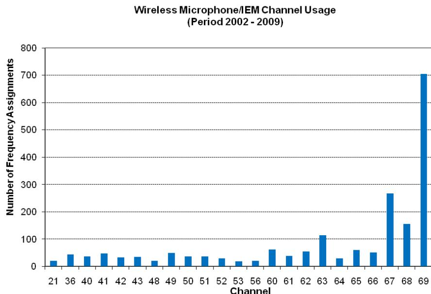
**Figure 5: Wireless Mics/IEMs Channel Usage Statistics (2002 - 2009)**
