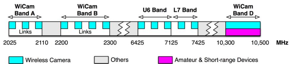
**Figure 7: Spectrum potentially available for Wireless Camera after 2.3 GHz auction**
