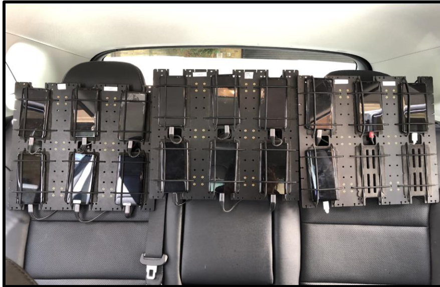
Figure 23: Measurement Set Up Showing Handsets.
