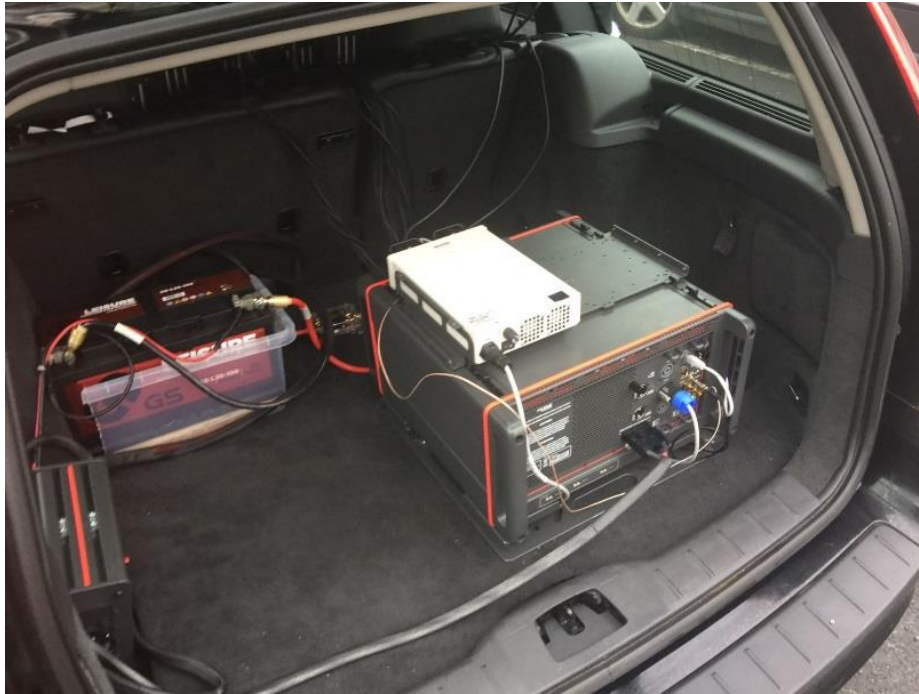
Figure 18: Nemo Invox, Connected to Handsets
