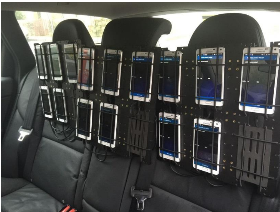
Figure 17: Measurement Set Up Showing Handsets
