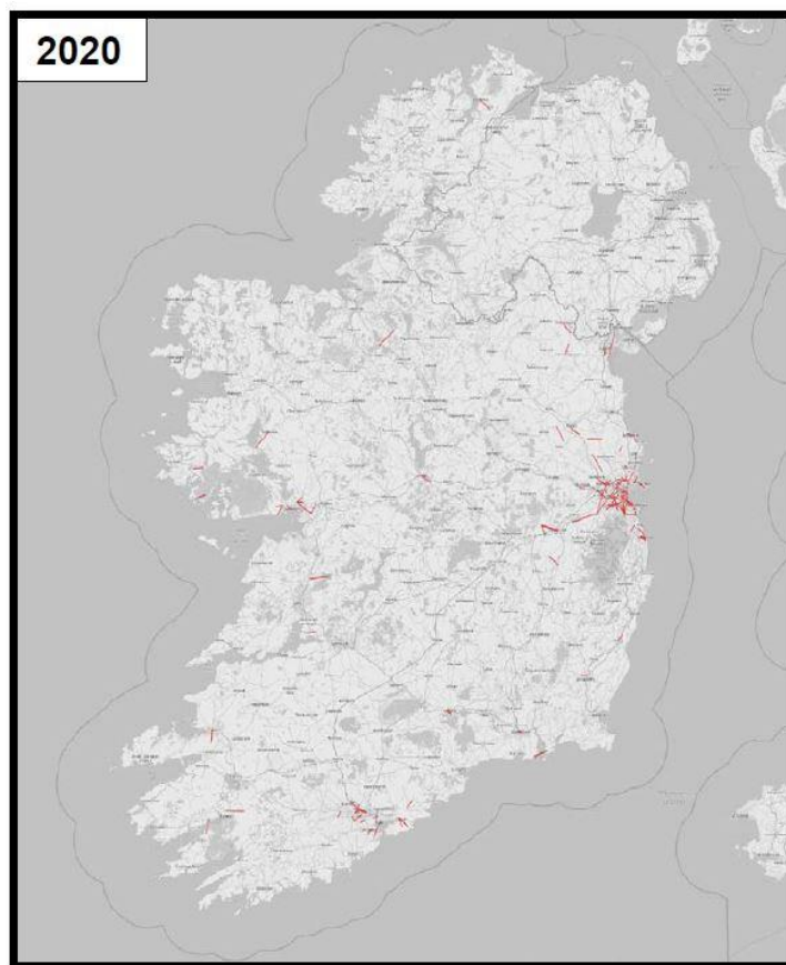
Figure 5.16: Fixed links operating in the 26 GHz band (Source: ComReg 20/109)
