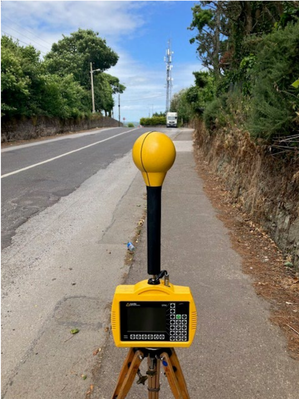
Photo 2. Frequency selective measurement location looking towards antennas
