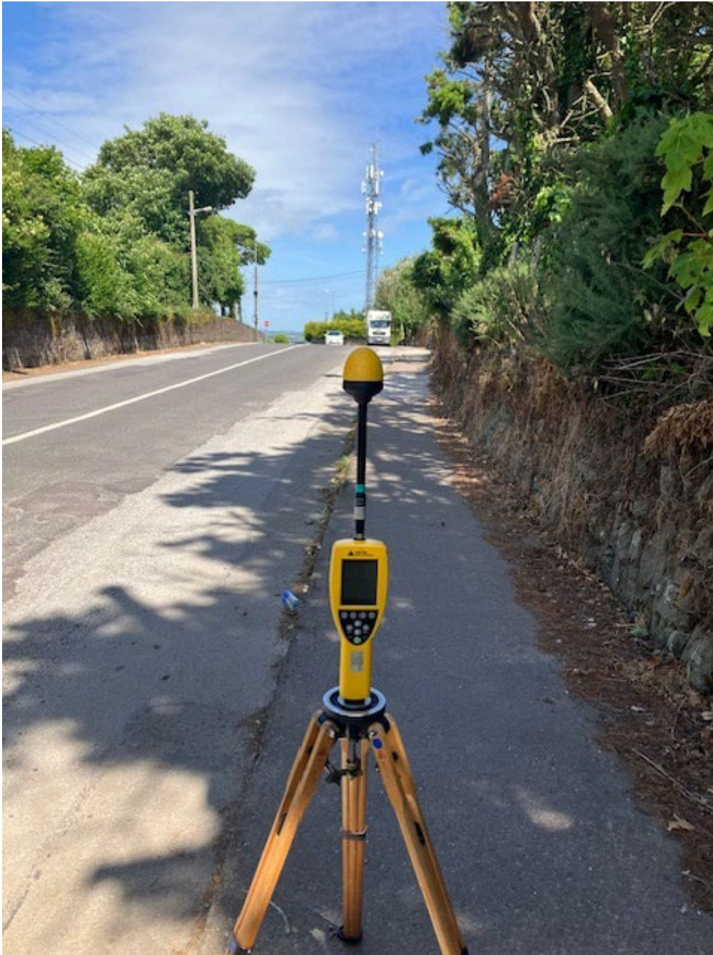
Photo 1. Broadband Measurement location looking towards antennas
