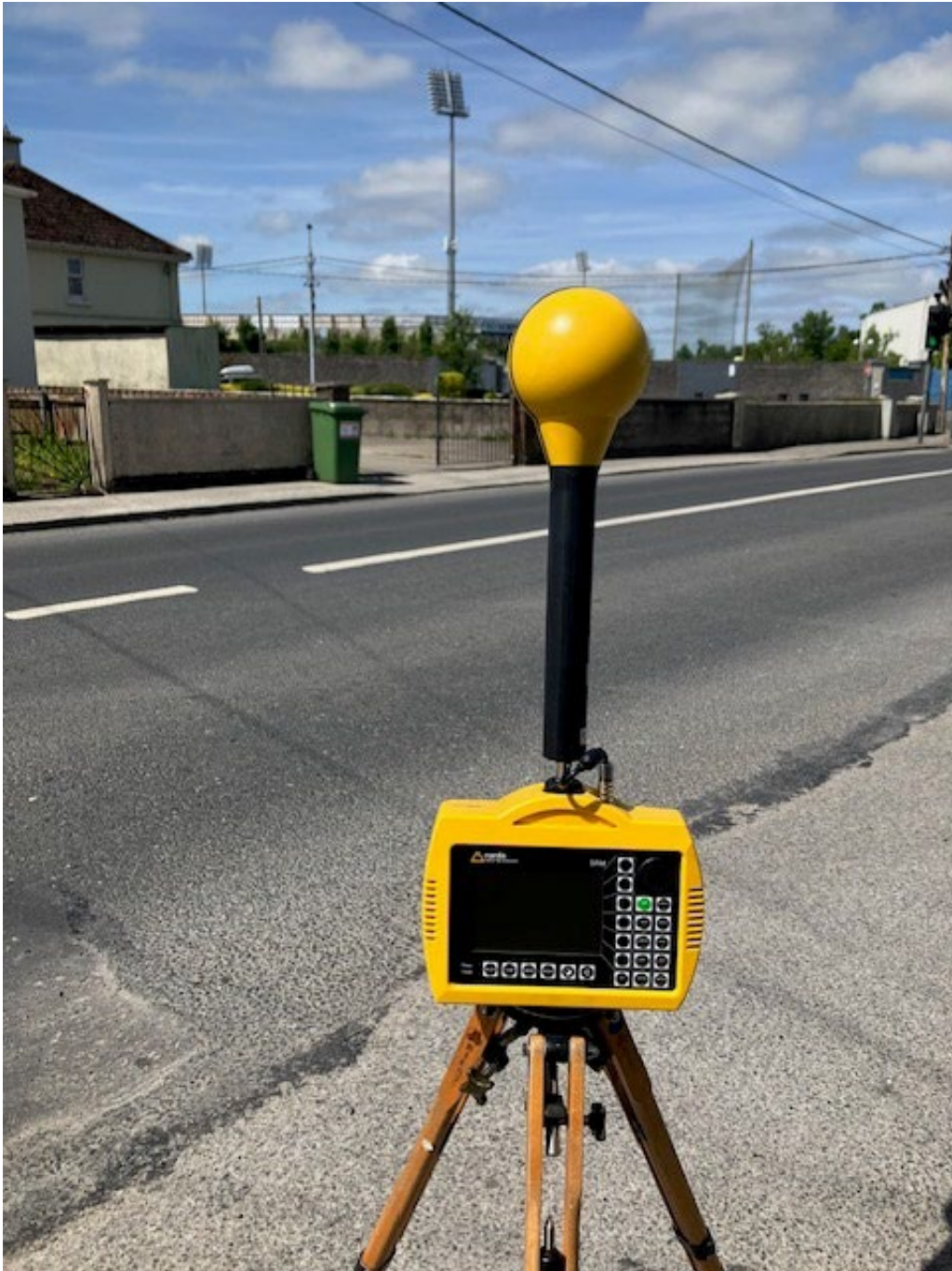
Photo 2. Frequency selective measurement location looking towards antennas
