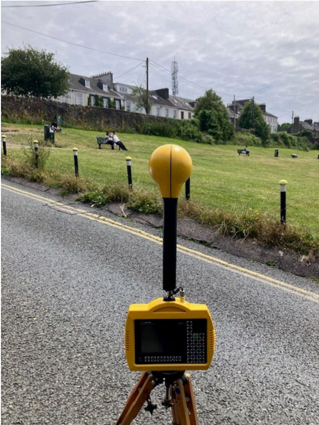
Photo 2. Frequency selective measurement location looking towards antennas
