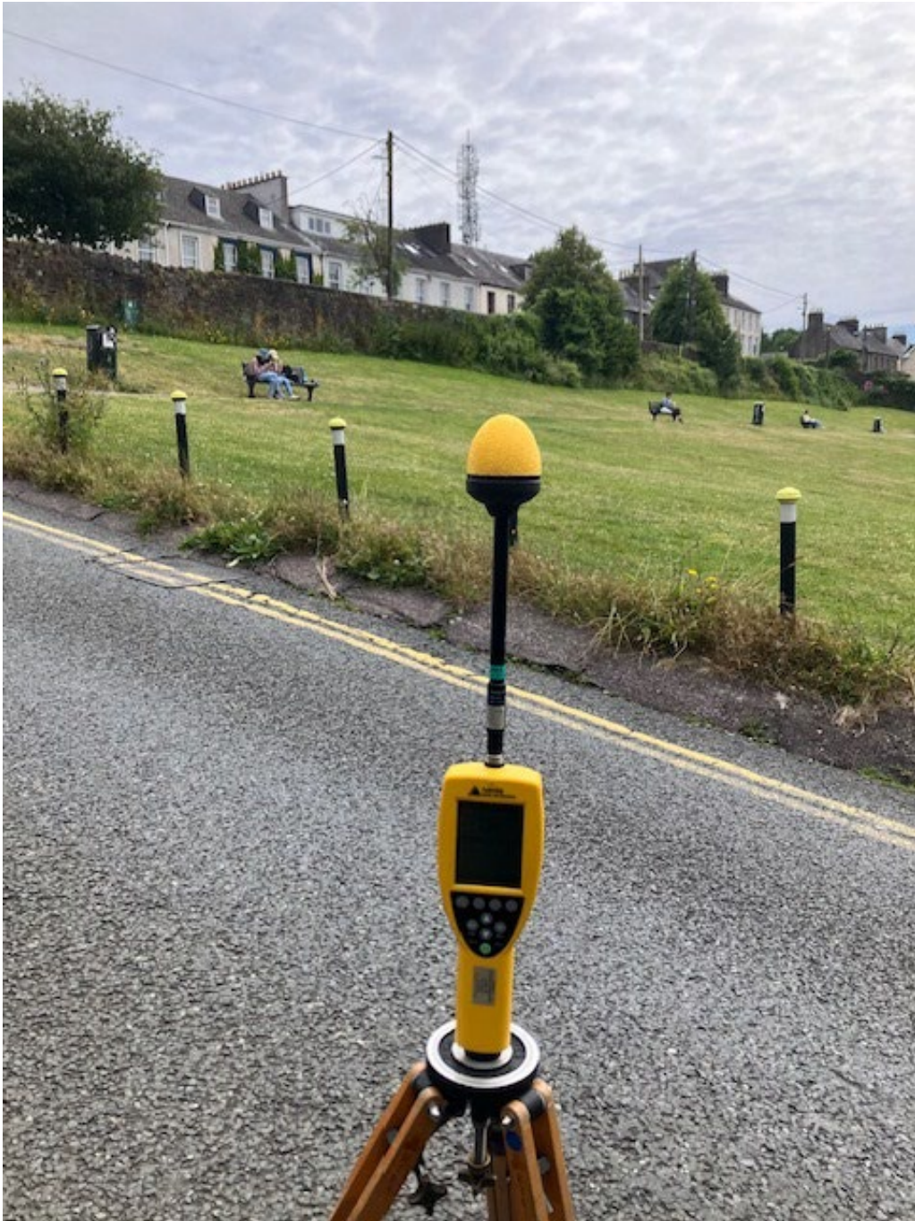
Photo 1. Broadband Measurement location looking towards antennas
