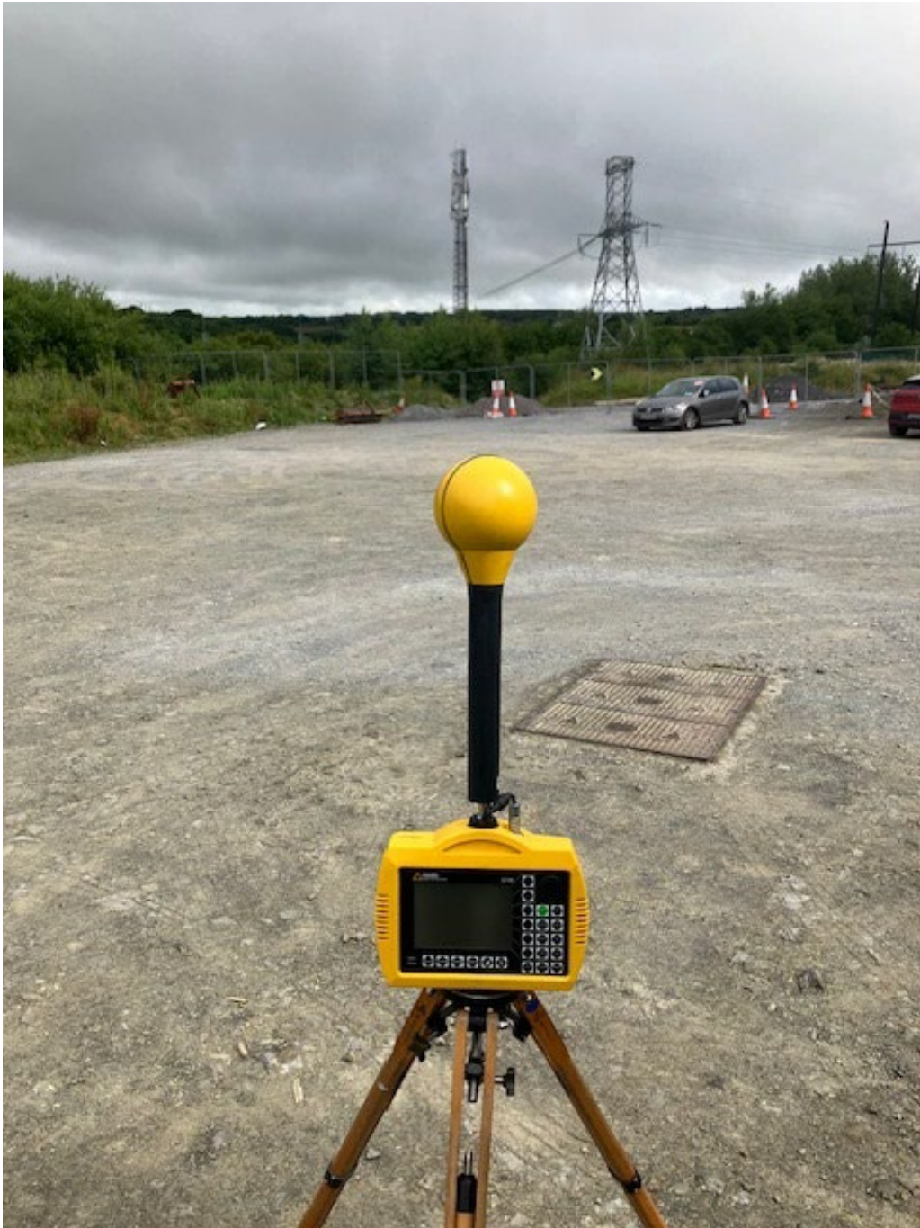
Photo 2. Frequency selective measurement location looking towards antennas
