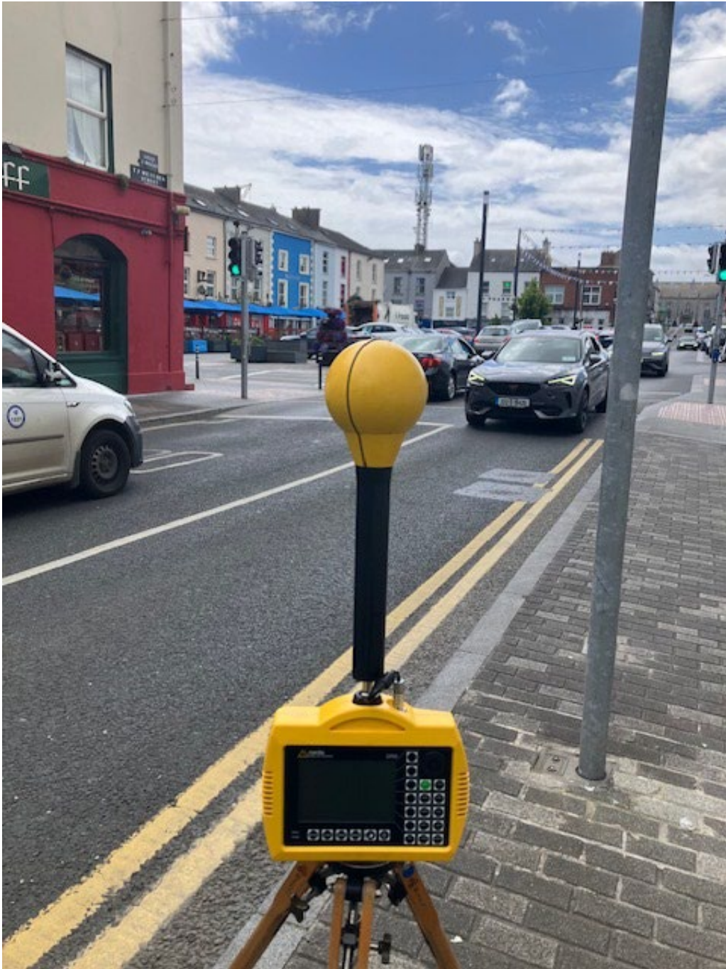
Photo 2. Frequency selective measurement location looking towards antennas
