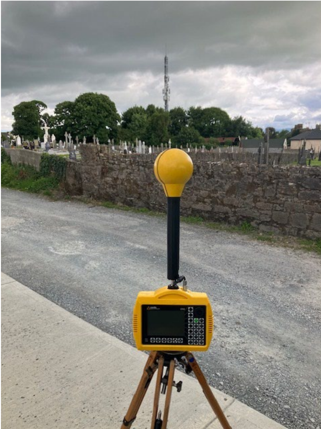
Photo 2. Frequency selective measurement location looking towards antennas
