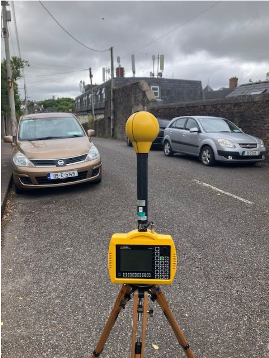
Photo 2. Frequency selective measurement location looking towards antennas
