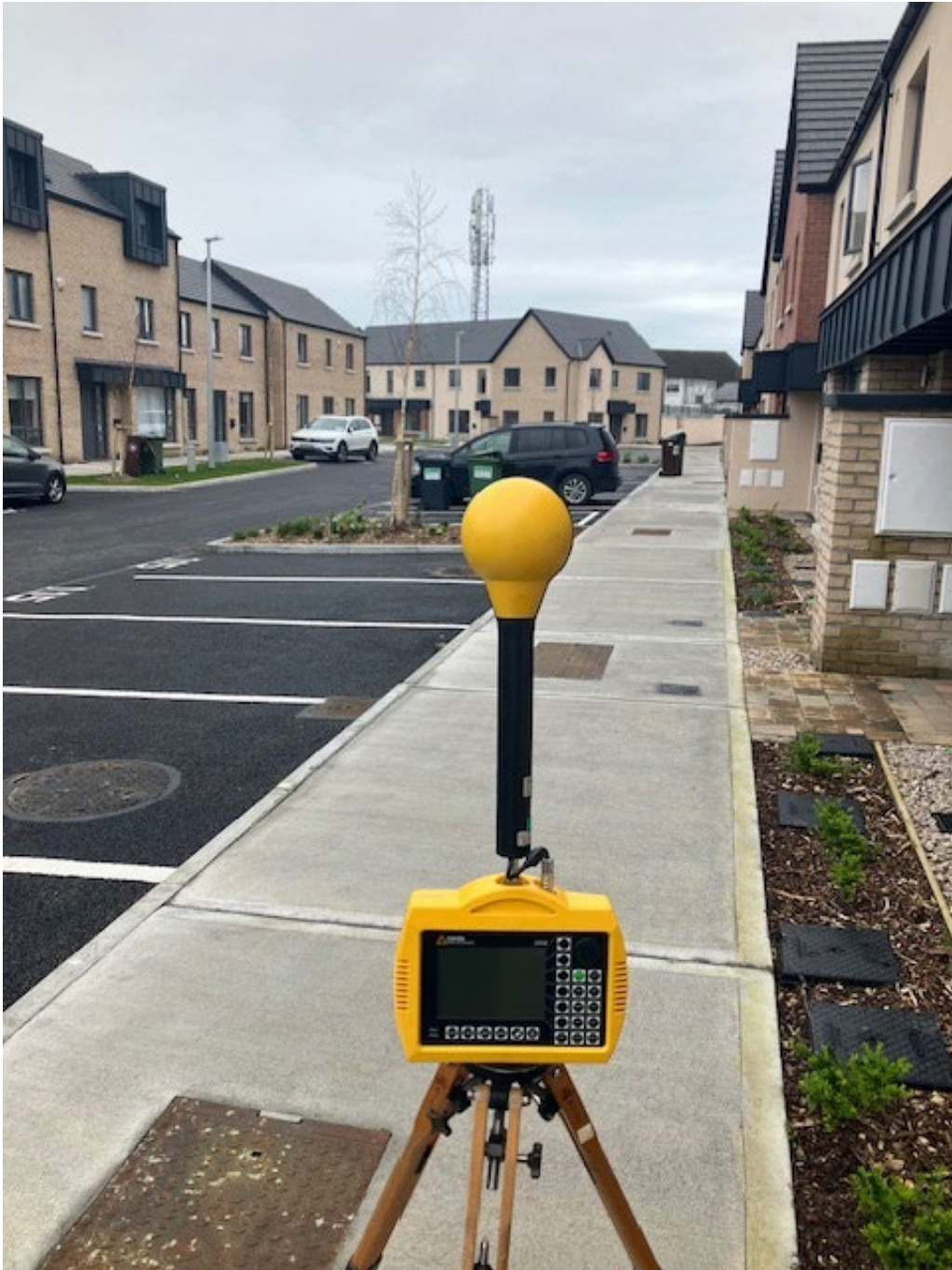
Photo 2. Frequency selective measurement location looking towards antennas
