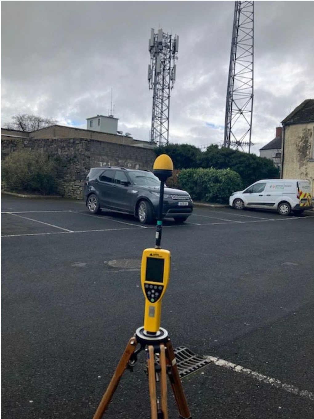
Photo 1. Broadband Measurement location looking towards antennas
