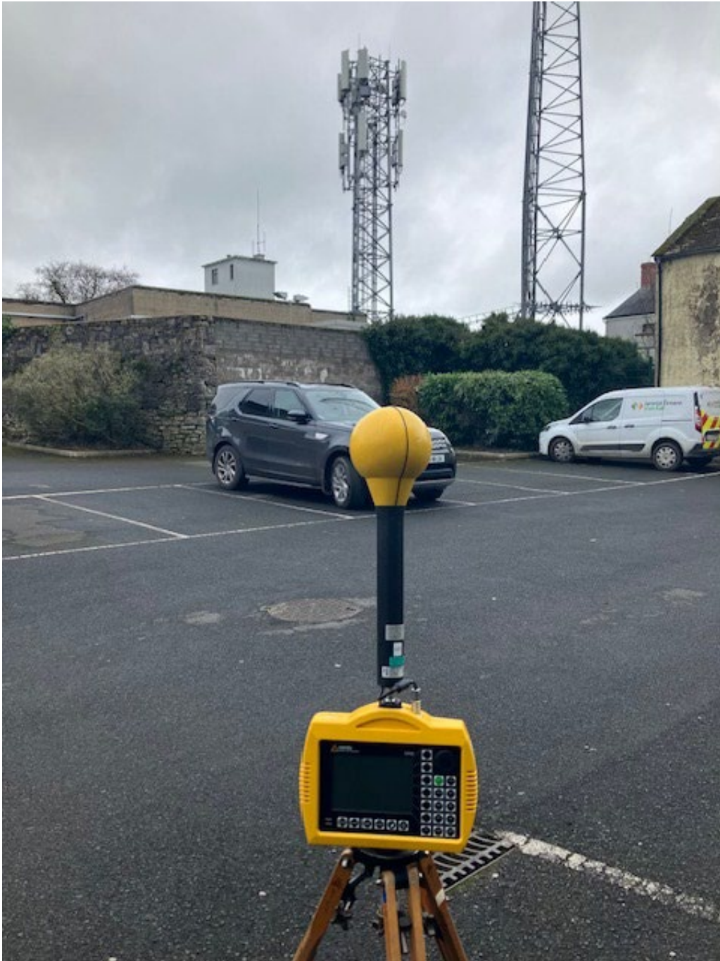
Photo 2. Frequency selective measurement location looking towards antennas
