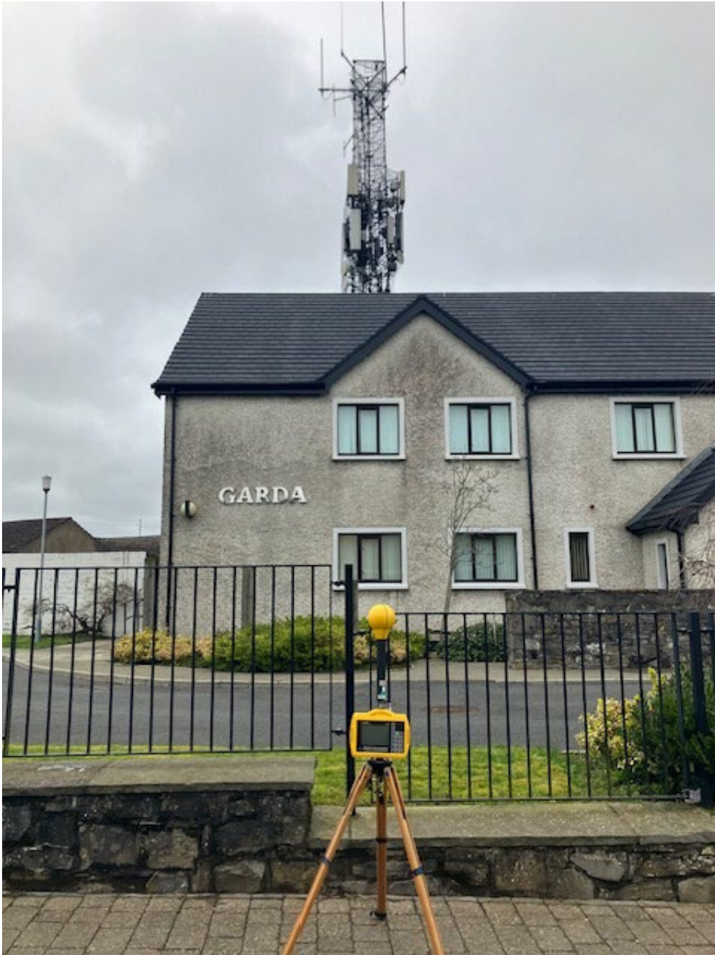
Photo 2. Frequency selective measurement location looking towards antennas
