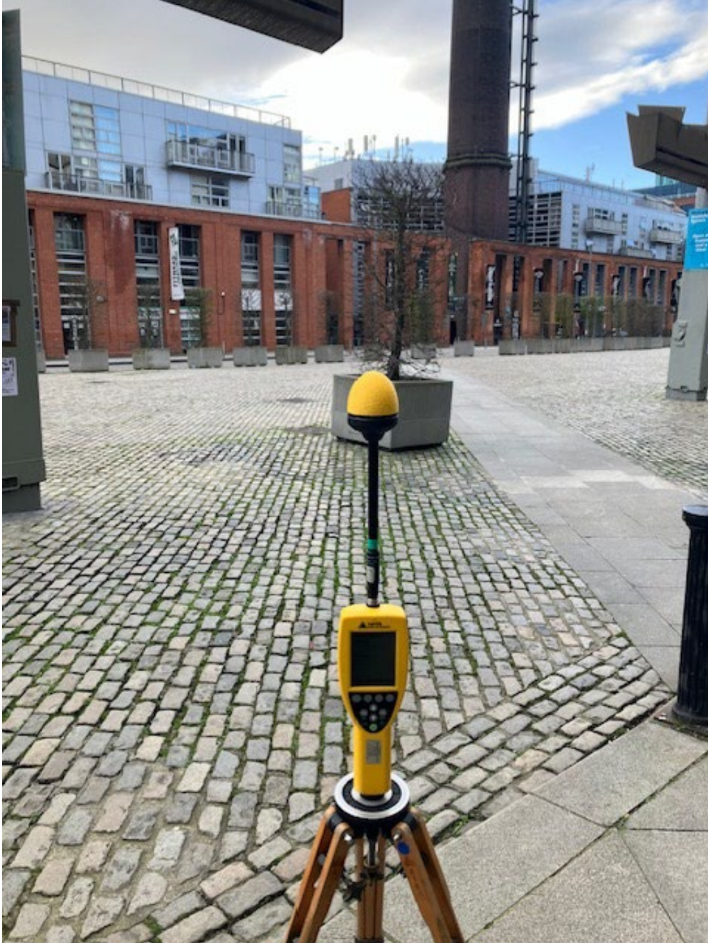
Photo 1. Broadband Measurement location looking towards antennas
