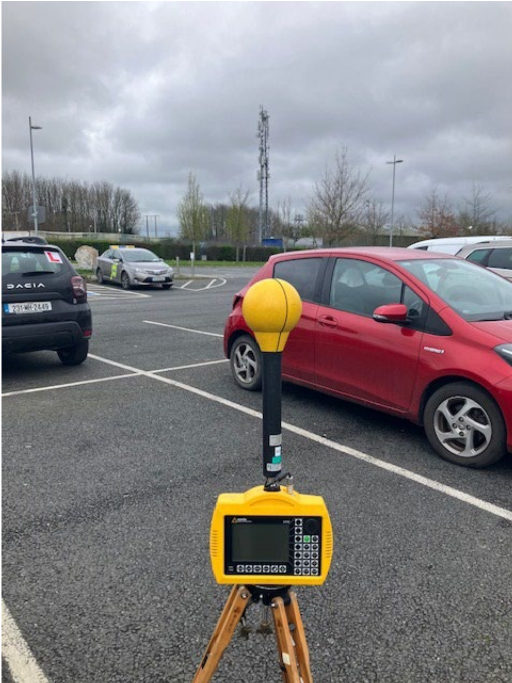
Photo 2. Frequency selective measurement location looking towards antennas
