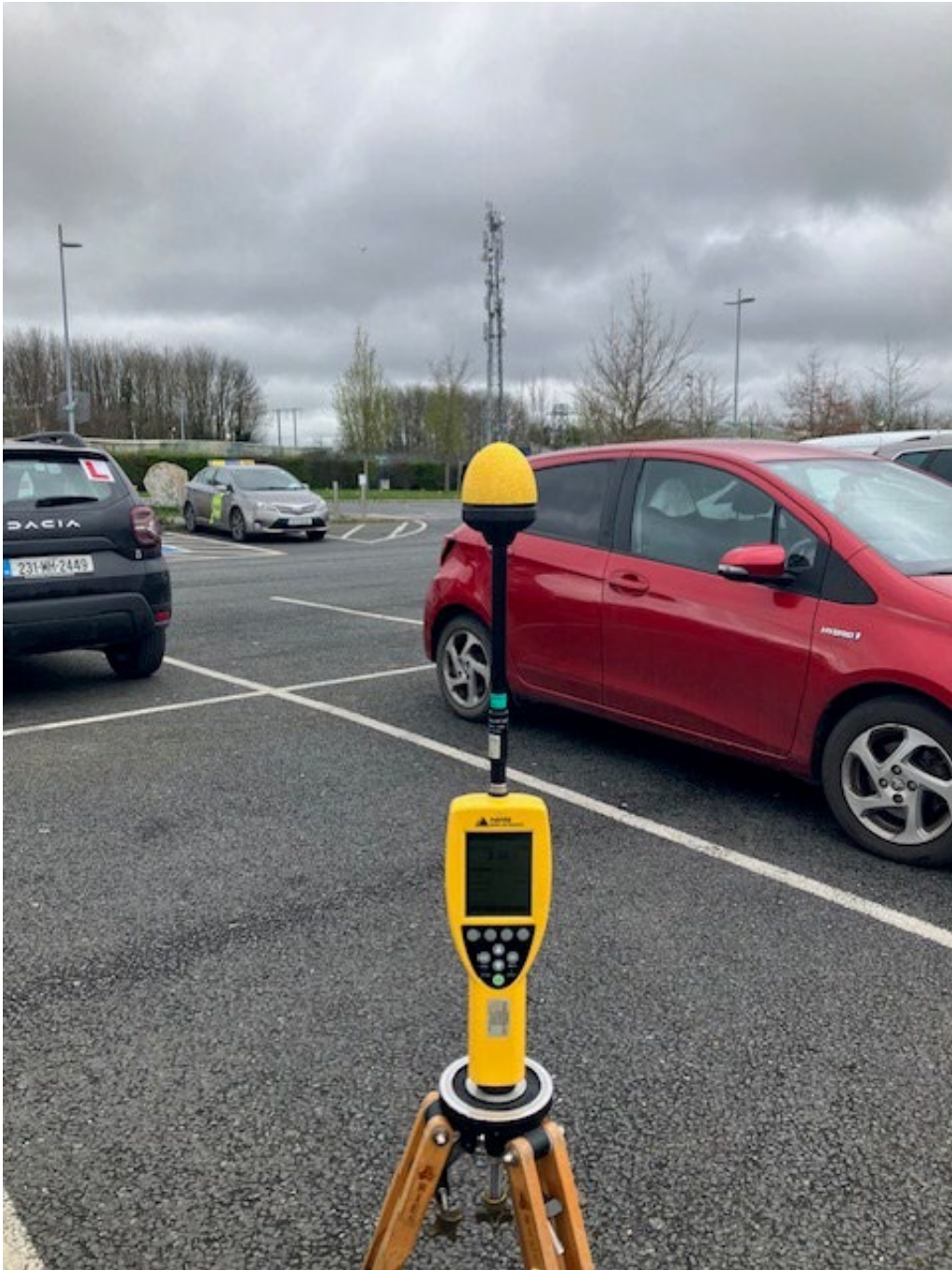
Photo 1. Broadband Measurement location looking towards antennas
