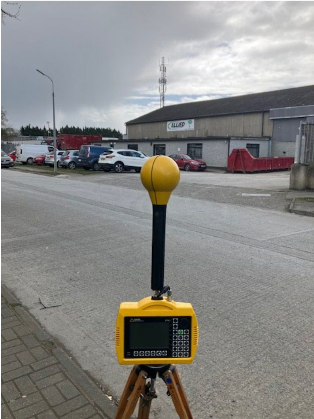
Photo 2. Frequency selective measurement location looking towards antennas
