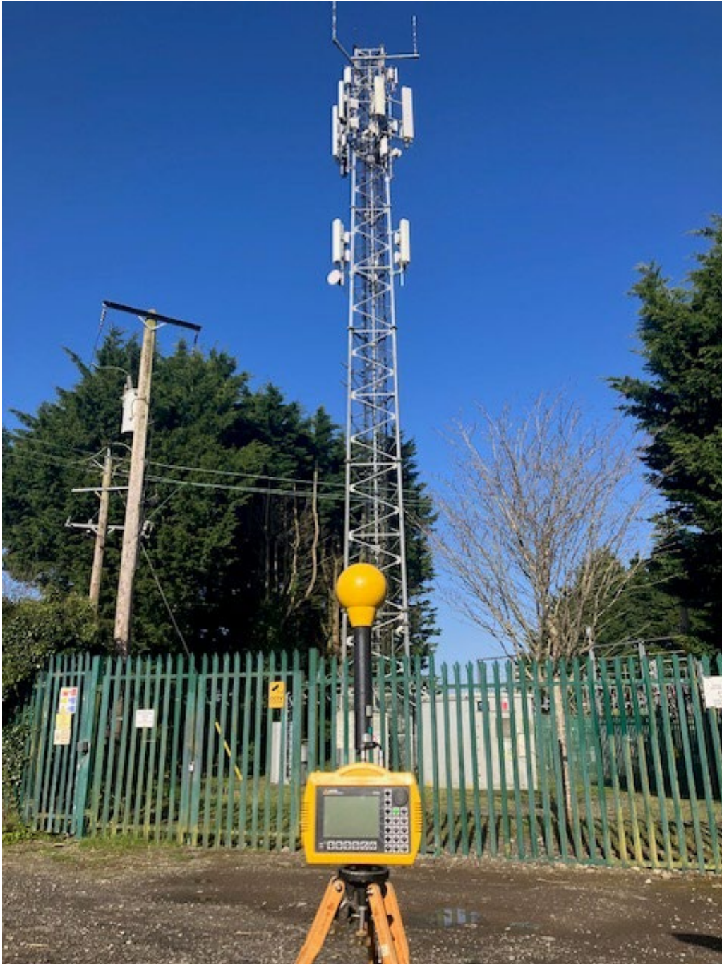
Photo 2. Frequency selective measurement location looking towards antennas
