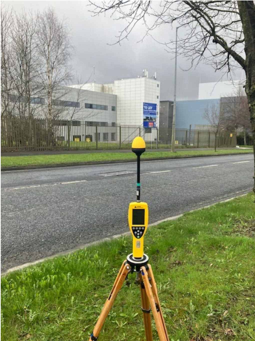
Photo 1. Broadband Measurement location looking towards antennas
