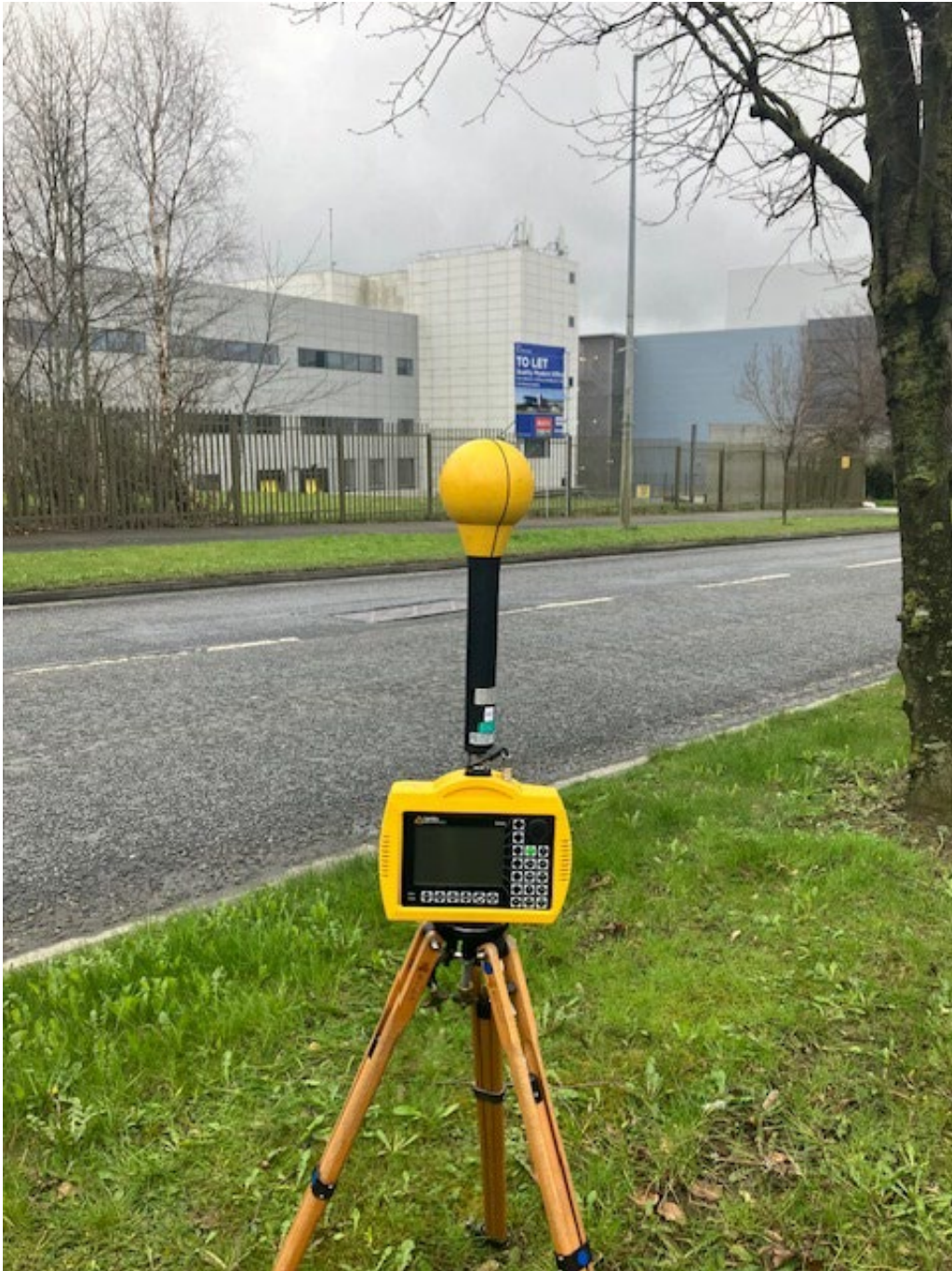
Photo 2. Frequency selective measurement location looking towards antennas
