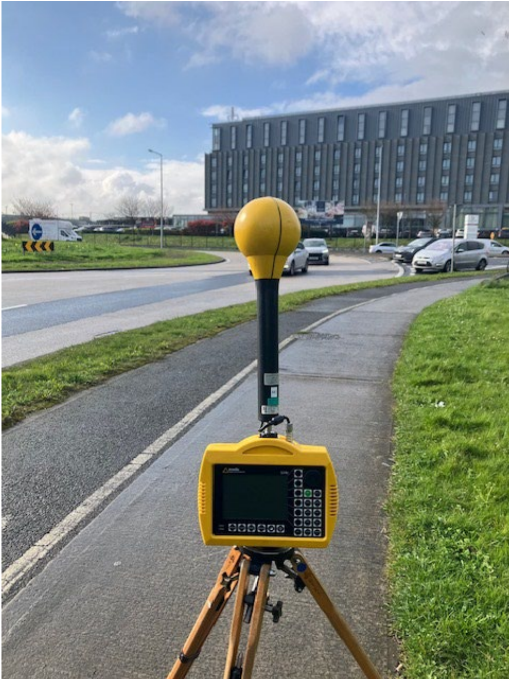
Photo 2. Frequency selective measurement location looking towards antennas
